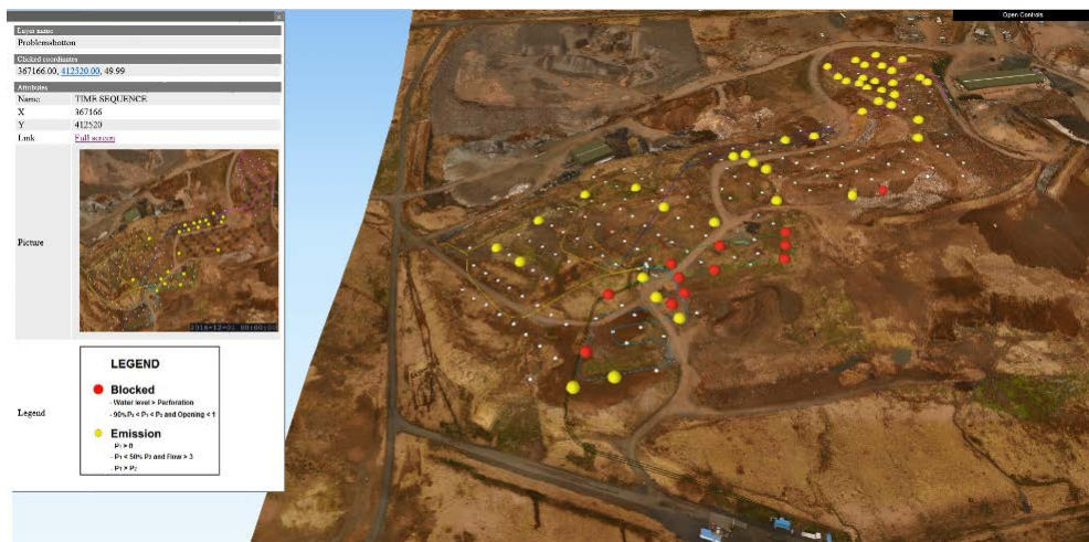
Fig. 4. 3D visualization of emissions and blockage issues. Red spheres correspond to blocked wells, while yellow spheres correspond to wells with excessive overpressure inside
