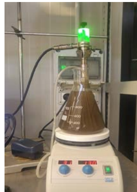
Fig. 2. SOUR experimental set-up.
