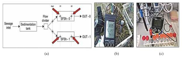
**Fig. 4.** Pilot plant scheme with measurement points for DO and pH and water level identified with red arrows (a). pH measurement system (b); Ion-Selective electrode for NH<sub>4</sub><sup>+</sup>-N measurement (c)
