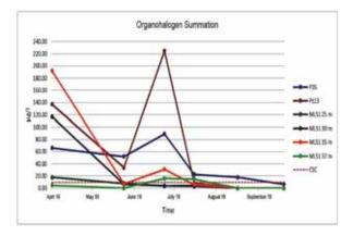
**Fig. 7**. Concentration trends for chlorinated ethylenes in groundwater at monitoring points in the treatment area, before and after EHC<sup>®</sup> L injections performed in May 2019
