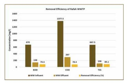
Fig. 3. Removal Efficiency of Rafah WWTP
