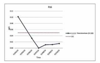
Fig. 10. Trend in R-130 concentrations in groundwater at the Pz6 monitoring point in the treatment area before and after EHC<sup>®</sup>L injection performed in May 2019
