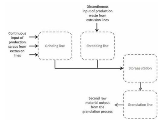
**Fig. 2.** Block diagram of the recycling compartment. Inputs are shown in black; processes are dotted and outputs are shown in gray
