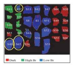
Fig. 7. Prediction map of the plastic validation set obtained after the application of the HI-PLSDA model. The plastic classes are dark colored, light colored with high Br (Br> 2000 mg/kg) and light colored with low Br (Br < 2000 mg/kg), corresponding to the red, green and blue particles, respectively. Samples circled in yellow (S40, S57 and S65) are incorrectly identified.
