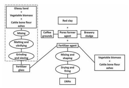
Fig. 1. Fertilizer glass and LWAs production process
