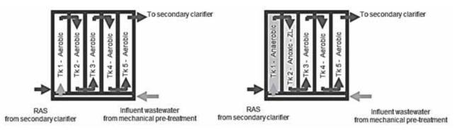
Fig. 1. Original configuration (on the left) and upgraded configuration (on the right) of biological process scheme in Line 1 at the YBSD wastewater treatment plant
