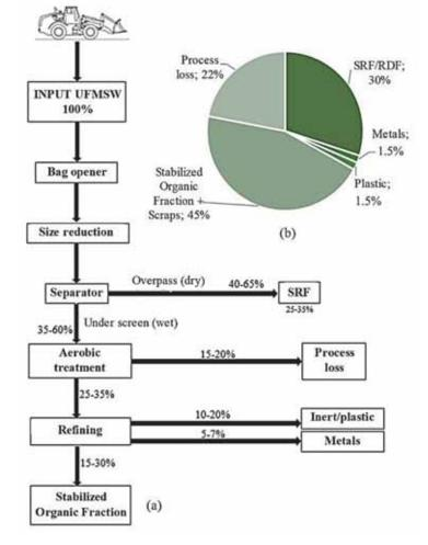
Fig. 3. MBT plant: (a) process diagram with mass balance; (b) typical output composition
