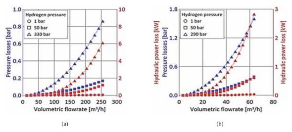
Fig. 2. (a) pressure drops and hydraulic power loss along the Sealine 1 crossed by hydrogen,(b) pressure drops and hydraulic power loss along the Sealine 2 crossed by hydrogen
