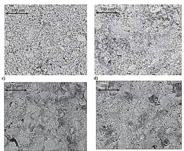
Fig. 3. ESEM analysis of LWAs (300x): a) B-Ash, b) C-Ash, c) B-Glass, d) C-Glass
