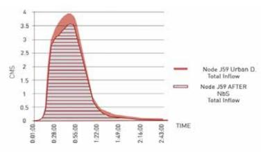
Fig. 11. NbS associated together vs Urban developed. Y-axis describes the surface runoff in cubic meters per second, while the X-axis describes the amount of time of the event, in this case is about 1 hr
