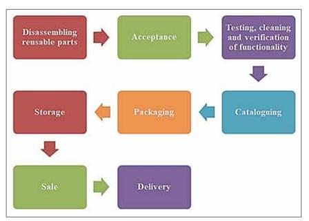
Fig. 4. Flow chart: original used spare parts line
