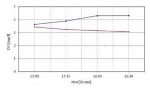
**Fig. 5.** HRT = 1.5 h - Dissolved Oxygen concentrations measured by YSI probe in S2 sampling tubes with plants (blue line) and without plants (red line)
