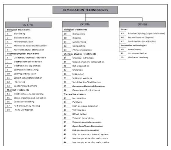
Fig. 2. Remediation technologies identified for in situ, ex situ and other types of technologies
