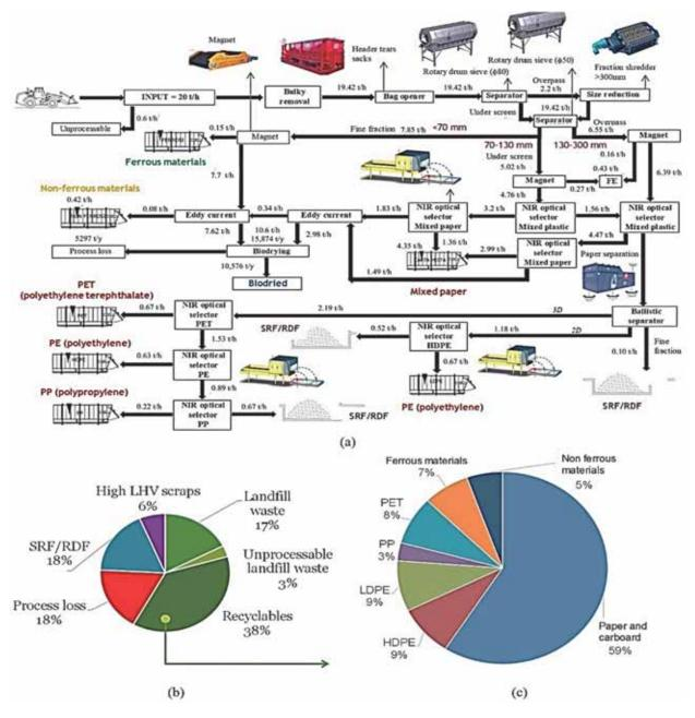
Fig. 2. SRMR plant: (a) process diagram with mass balance; (b) typical output composition; (c) potentially recoverable materials
