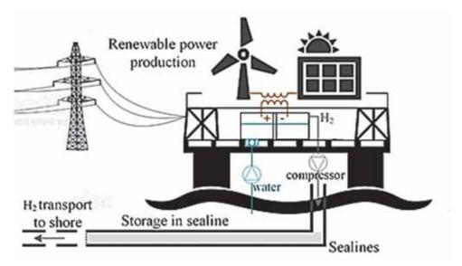
Fig. 1. Layout of the hypothesized integrated energy system.
