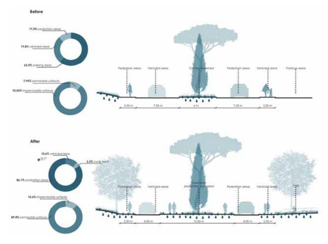
Fig. 9. Section of permeable surface before and after the project and comparison of the difference in permeability. In this case with the project there is an 80% increase of permeable surface.
