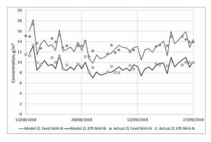
Fig. 6. Validation of the YBSD MABR model in Biowin on influent and effluent ammonia concentration in the MABR zone
