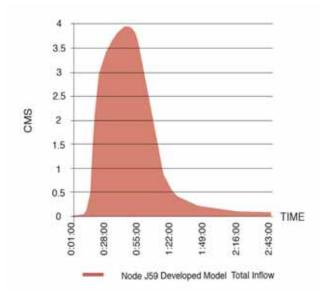
Fig. 6. Graph of the Urban developed runoff, the total flow volume is 3.94 (CMS/hr). Y-axis describes the surface runoff in cubic meters per second, while the X-axis describes the amount of time of the event, in this case is around 1 hr
