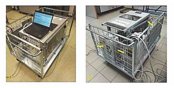
Fig. 9. BIOWYSE support equipment for field tests. a) PC tool, b) power supply, chiller and fluidic panel
