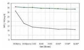
**Fig. 10.** HRT= 30 h - Ammonium concentration (NH<sub>4</sub><sup>+</sup>-N) analysed in samples from S2 sampling tubes without plants (green line) and with plants (grey line).\*day after
