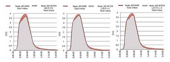
**Fig. 12.** First graphic: combination of Draining parking lots and Green roofs - reduction of surface runoff to 3.63 cubic meters per second / hr (- 7.9%); Second graphic: combination of Draining parking and Water tanks - reduction of surface runoff to 3.75 cubic meters per second / hr (- 4.9%); Third graphic: combination of Green roofs and Water tanks- reduction of surface runoff to 3.68 cubic meters per second / hr (- 6.8%).
