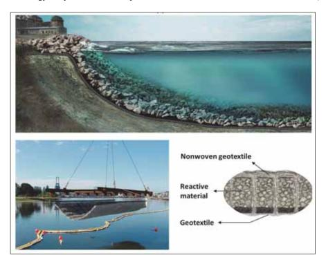
Fig. 4. Examples of full-scale amendments capping applications and schematic of reactive core mat (Huesker, 2020; Mineralstech, 2020)
