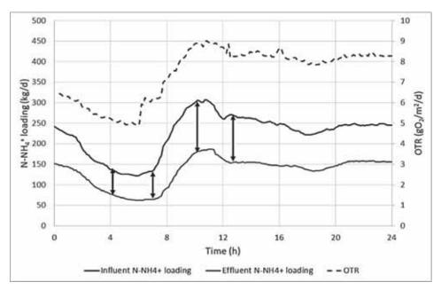
Fig. 4. Calculated OTR and influent and effluent ammonia loading to/from the MABR zone
