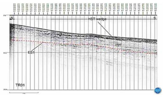
Fig. 4. CHIRP seismic profile running perpendicular to the High Stand (HST) sediment wedge in proximity of the Azalea A platform. ES1 is the subaerial erosional surface related to the last sea level low stand, occurred approximately 20,000 years ago and TST (Transgressive System Tract) is the sediment sequence deposited during the last sea level rise which culminated in the current high stand of the sea level around 6,000 years ago
