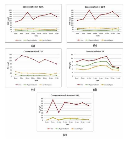
Fig. 8. Concentrations [mg/L] of the physico-chemical parameters at the different sampling points: (a) BOD<sub>5</sub>, (b) COD, (c) TSS, (d) TP (e) NH<sub>4</sub>
