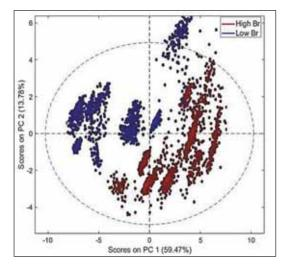
Fig. 6. PC1-PC2 score plot of the plastic samples constituting the training set for the two groups characterized by the presence of high (Br> 2000 mg/kg) and low (Br < 2000 mg/kg) bromine content
