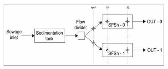
Fig. 2. Flow scheme implemented in the pilot plant during measurements campaigns
