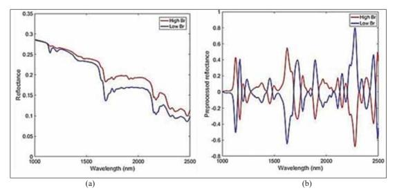
Fig. 5. Average raw reflectance spectra: (a) and average pre-processed reflectance spectra; (b) of the plastic waste samples acquired by HSI in the wavelength range 1000-2500 nm, representative of the two classes characterized by high (Br> 2000 mg/kg and low (Br < 2000 mg/kg) bromine content
