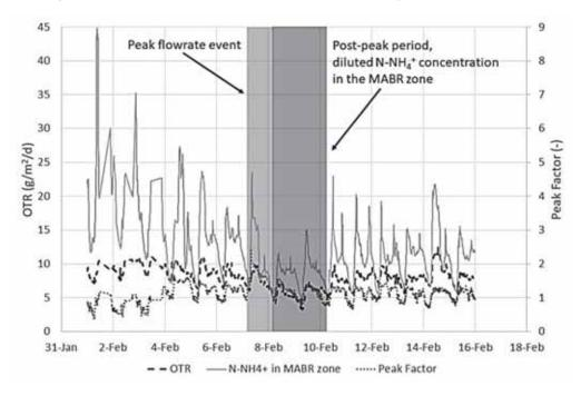
Fig. 5. Impact of rainy weather conditions on the OTR. The peak event (flow up to 2.4 times the average flow value) in the light grey area, the ammonia dilution effect in the MABR zone in the dark grey area
