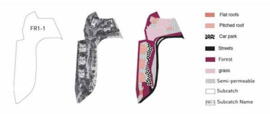
Fig. 5. Example of the investigation process of permeability that was made for each sub-catchment
