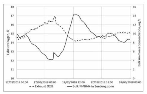
Fig. 3. Typical daily pattern of oxygen concentration in the exhaust air and ammonia concentration in the mixed liquor in the MABR zone
