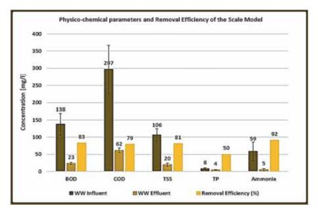
Fig. 9. Influent and effluent at the scale-plant: average values
