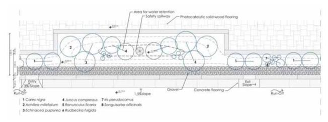
Fig. 8. Bioswales detail. Phyto-depuration plant and system operation for the collection of rainwater
