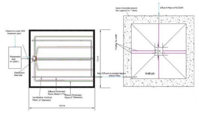
Fig. 6. Plant and dimensions of scale model design
