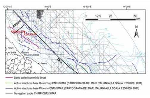
Fig. 3. Bathymetric contour map showing the location of the Azalea A platform in respect to the city of Rimini, the deep-buried Apenninic thrusts and 2 single channel seismic reflection profiles (CHIRP) and displayed as an example in Fig. 4
