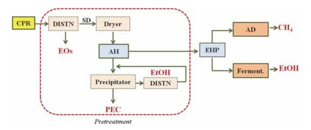
**Fig. 2.** Biorefinery strategy for CPR valorization. Based on Patsalou et al., 2019. (AD=anaerobic digestion; AH=acid hydrolysis; CH<sub>4</sub> = Methane; DISTN= distillation; EHP= enzymatic hydrolysis procedures; EtOH= ethanol; Ferment=fermentation; PEC=pectins; SD=solid fraction)
