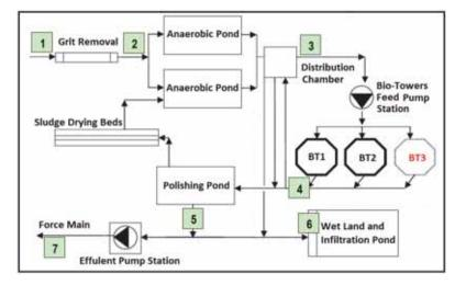
Fig. 2. General Layout of Rafah WWTP (ICRC, 2013)
