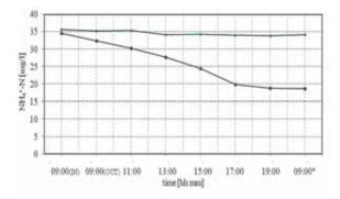
**Fig. 8.** HRT= 12 h - Ammonium concentration (NH4<sup>+</sup>-N) analysed in samples from S2 sampling tubes without plants (green line) and with plants (grey line).\*day after
