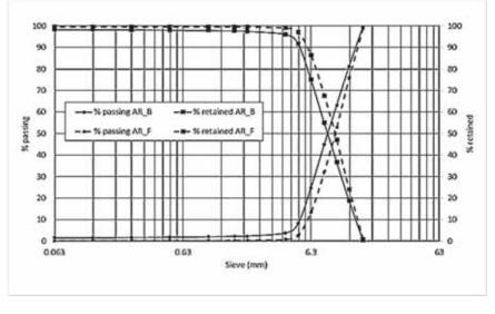
Fig. 3. Particle size distributions of recycled aggregates
