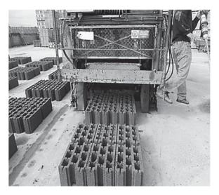
Fig. 5. Production of recycled concrete blocks
