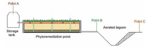
Fig. 5. Sampling points in the scale-pilot plant
