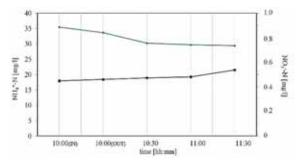
Fig. 6. HRT= 1.5 h - Ammonium (green line) and Nitrate (black line) concentrations in samples from S2 tubes
